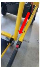
2. Pull out bolt. Nut between handrail and frame may need to be turned in order to release the bolt.
