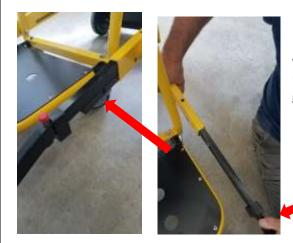
4. When handrail is extended you will notice a black insert under the rail (illustration 1). Pull hard while depressing the red release button and the guiderail will come out of frame channel. (illustration 2)
