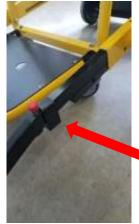
3. Once bolt is removed, telescoping handle will no longer be fixed to the frame. Push red release button (illustration 1). Remove plastic cap covering end of frame (illustration 2). Slide out handrail.
