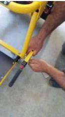
1. Remove top bolt with Allen wrench on outside of bolt (red arrow) and adjustable wrench on nut on inside of chairs frame (blue arrow)
