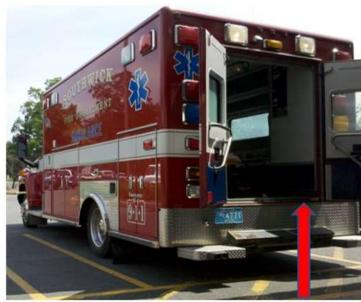
Maximum Loading Height Measured From Ground to Loading Platform
