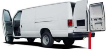
Maximum Loading Height Measured From Ground to Loading Platform
